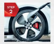
Hose or jet wash your wheels and wheel arch liners to remove as much loose dirt as possible. If your rims and arches are still coated with dirt and, or brake dust, reapply the Iron Removing Wheel & Paint Cleaner and agitate the dirty areas with the appropriate brushes. Namely a soft detail brush for wheel nuts, a soft wheel brush for rims and a long handled wheel arch brush for your wheel arches. And then rinse with a hose or jet wash.
